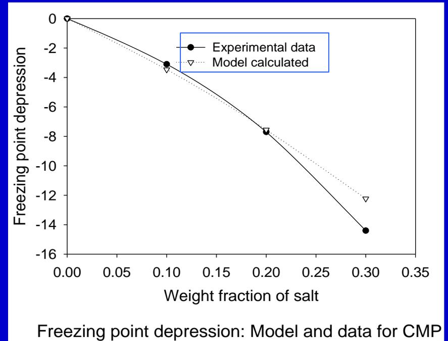
Freezing point depression model predictions for CMA and CMP (Ca:Mg 3:7)
