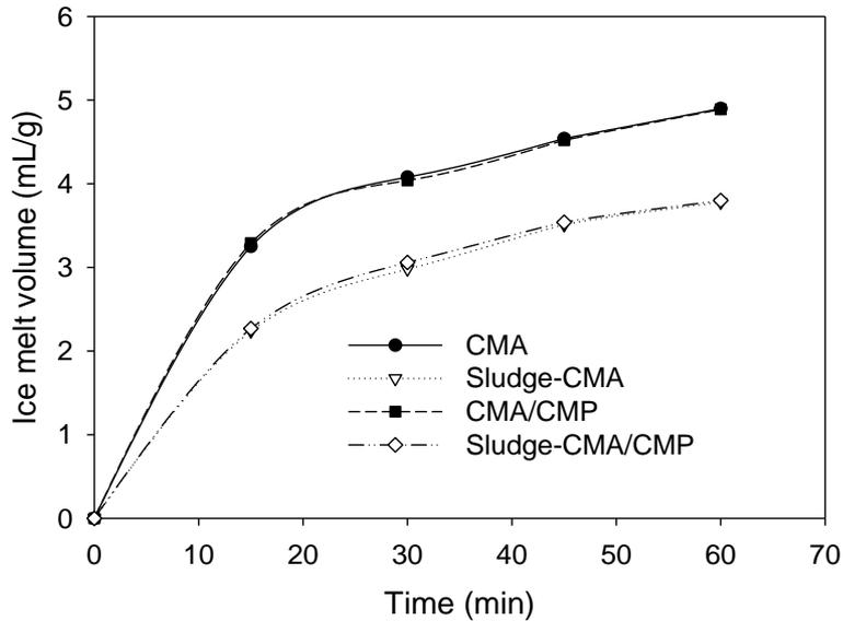
Ice melting rates CMA/CMP and sludge-deicer at -7 C
