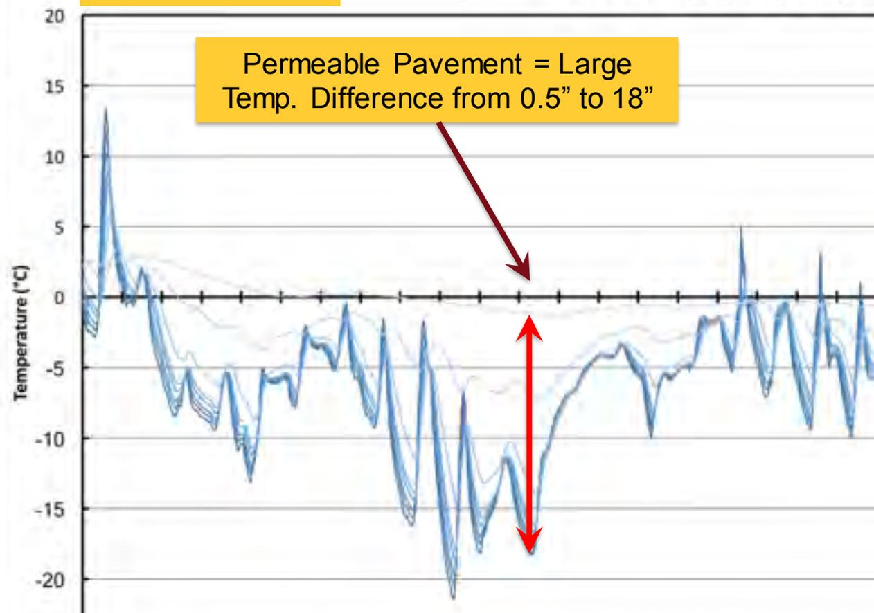
**Bottom Line: Permeable Pavements are Insulating!**
